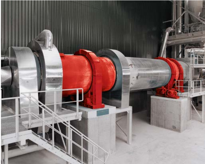
Rotary tubular calciner with integrated cooler
