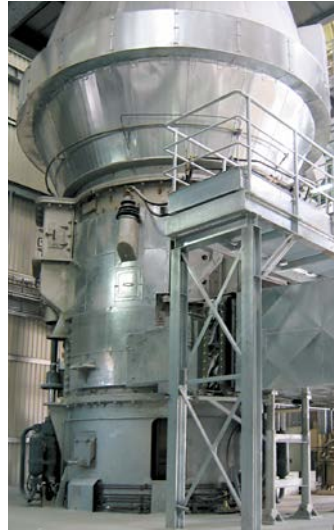
Ring-roller mill for drying or mill calcining
